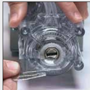
3. Reassemble two halves and mount on drive.
