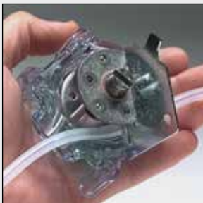
1. Disassemble pump head. Load tubing.
