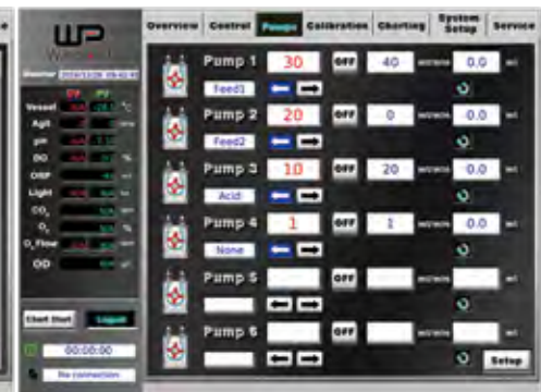
Pumps Control speed, direction, total volume and flow rate
