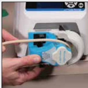
2. Place tubing over rollers and through retainers.
