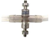
Optical Couplers Installed to Flow Cell
